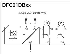
Connect the power supply to the terminals A1 and A2 or A3 and A2.
