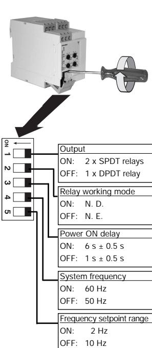
To access the DIP switches open the grey plastic cover as shown on the left.
