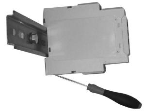
Hang the device to the DIN-rail being sure that the spring closes. Use a screwdriver to remove the product as shown in figure.
