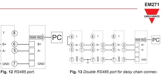
Fig. 13 Double RS485 port for daisy chain connection.
