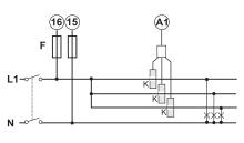
Fig. 7 One-phase system, three single-phase loads.
