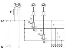
Fig. 8 One-phase system, six single-phase loads.
