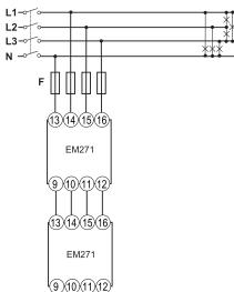
Fig. 4 Three-phase system, three single-phase loads.
