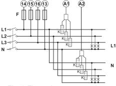
Fig. 6 Three-phase system, six single-phase loads.
