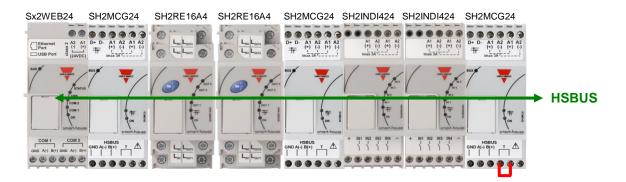
Also in this case there is no need to wire the RS485 for the HS speed bus since the local bus connector of the Dupline® modules is transparent to it. The installer only has to terminate the HS speed bus in the last bus generator of the RS485 network.
