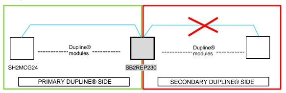
As soon as the short circuit is removed, the secondary side will automatically become operational again.
