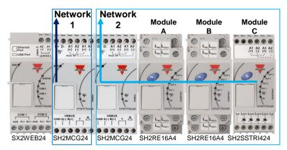
Modules A, B, and C are connected to the Dupline® network 2.
