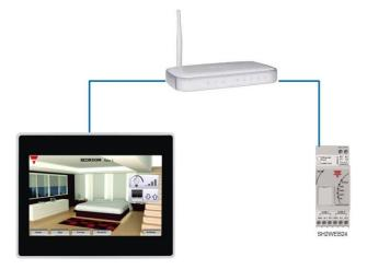
The TCP/IP devices can be connected to the Sx2WEB24 via a router by using both DHCP addressing or fixed IP with NAT forwarding if the Sx2WEB24 is to be visualised via the Internet.
