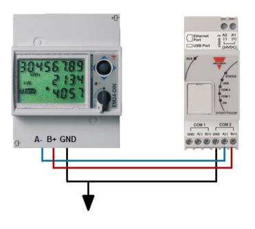
Different types of energy meter can be mixed, and they can also have different baud rate (see the Sx tool software manual for more details about how to configure the Sx2WEB24 to manage them).
