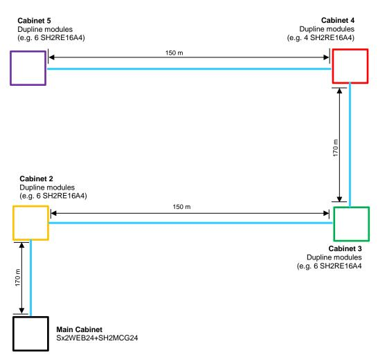
This network design is not recommended because the cable resistance and the load from bus-powered modules result in an excess of voltage drop.
