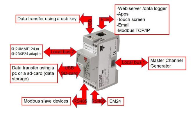
Here below a diagram of the system is shown.
