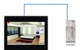
The TCP/IP device can be connected directly to the Sx2WEB24 with a peer to peer connection by using fixed IP (see the Sx tool manual to configure a fixed IP).
