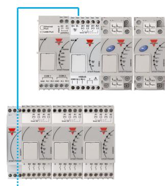
This connection must be avoided otherwise two Dupline® networks will be short circuited. If this should happen, the system will not be damaged since the bus is protected, but it will not work properly.
