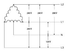
Fig. 4 Two-phase system with neutral (3-wire)
